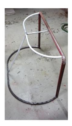
1. This Goal frame has been stripped of its netting; followed by the replacement of the lower metal fame piece that sits on the ice. After all the welds are done, the paint was stripped down with a wire wheel to bare metal so the new paint looks smooth and brand new.
