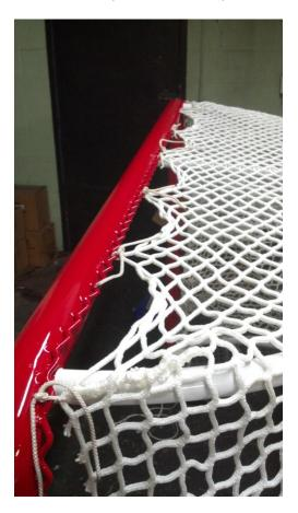
7. Goal netting is laid over the frame and tied off at about one foot intervals. This is done to make sure the net lays center to the frame, which makes tying the net that much easier.
