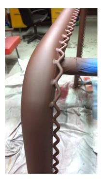
3. When painting a goal frame with the standard two colors, a nice seam must be made between them. That is done with blue painters tape to make a clean edge, followed by newspapers covering the majority of the fresh white paint. When the white is completely covered and protected, a coat of darker primer, in this case, brown, is sprayed down before the color coat.
